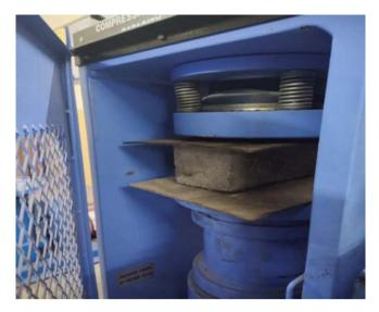
Fig. 8. Compression Test on brick Specimen.
