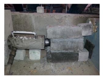
Fig. 15. Test setup for shear bond strength.
