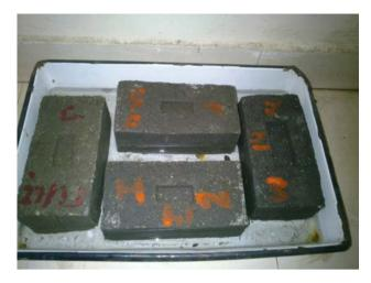
Fig. 9. Efflorescence test.
