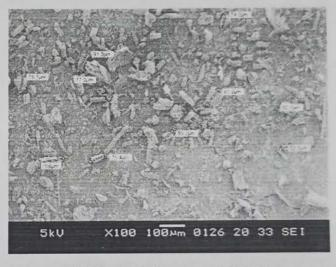
Fig. 2. Scanning electron micrographs for SCBA.
