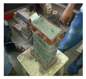
Fig. 17. Test setup for flexure bond strength.
