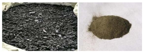
Fig. 2. (a) Cupola Slag before sieving (b) Cupola Slag after sieving.
