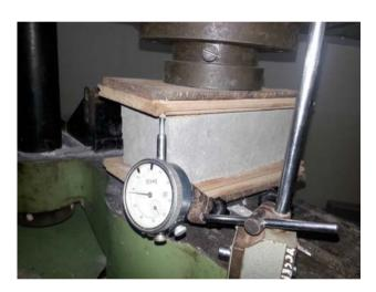
Fig. 13. Test setup for compressive strength.
