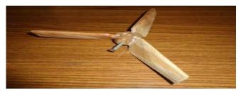
Fig. 4. Manufactured wooden NREL S809 aerofoil blade
