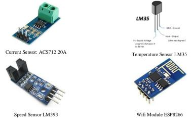
While that of wifi module ESP8266 is connected to the digital output pins of the microcontroller.
