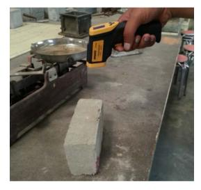
Fig. 11. Measurement of temperature by temperature gun.
