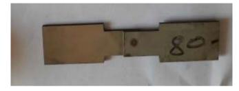
Fig. 2. Tensile test specimen according to ASTM E8 standard.
