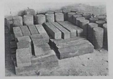
Fig. 7. The photo Cube. Beam and Cylinder prepared.
