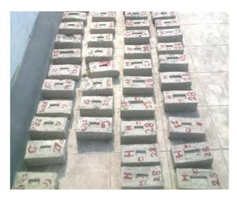
Fig. 5. Manufactured bricks kept for sun drying.
