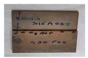
Fig. 1. 316L ASS and 430 FSS Dissimilar spot-welded plates.
