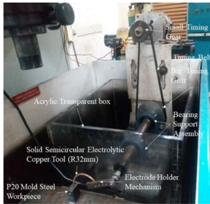
Figure 3 Actual experimental setup for curve machining
