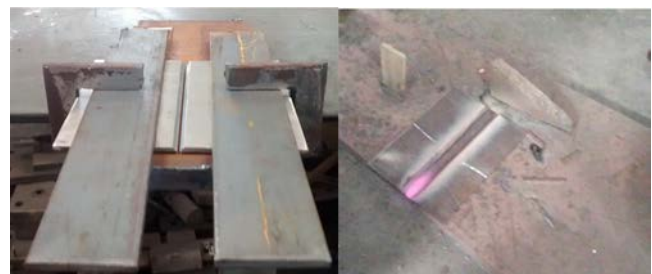
Figure 1 Welding plate fixture and welded plate
