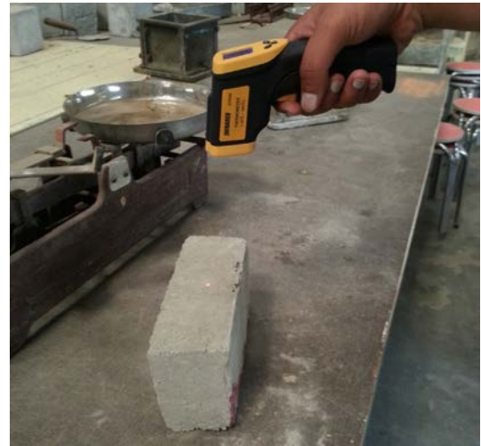
Fig. 11. Measurement of temperature by temperature gun.
