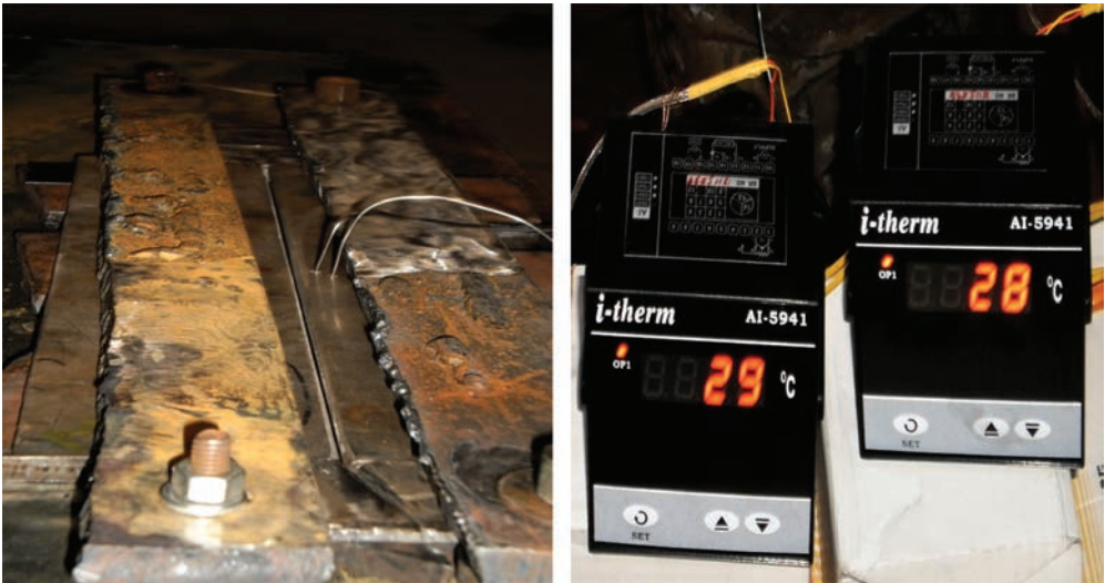
Figure 3. K-type thermocouple located at 3 mm and 7 mm from weld and temperature controller.
