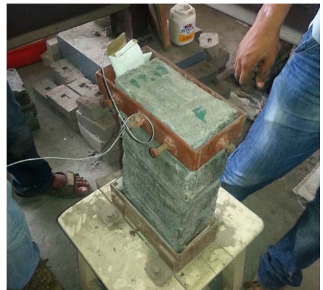
Fig. 17. Test setup for flexure bond strength.
