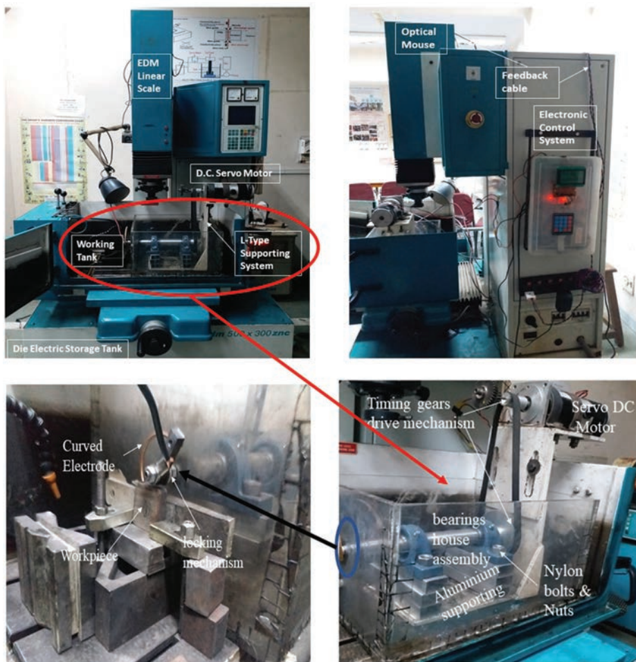
Figure 1. Experimental setup for curved machining EDM process
