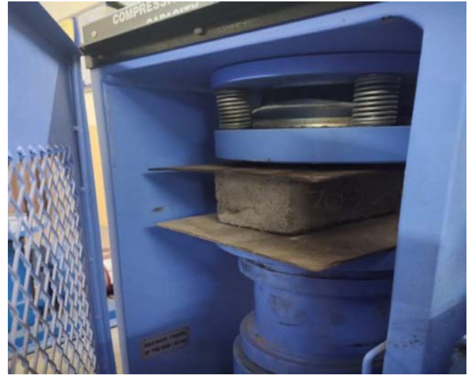
Fig. 8. Compression Test on brick Specimen.
