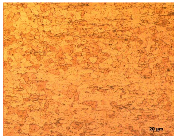
Figure 3 Microstructure of as received (AR) test steel
